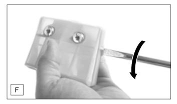
Pry apart the top and bottom of the air filter as shown in Figure F.
